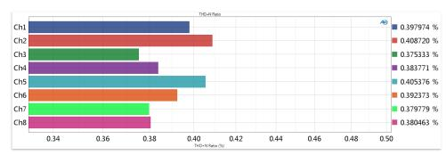
APx 585 and 586 are true multichannel analyzers; shown above is an 8-channel THD+N Ratio measurement.
